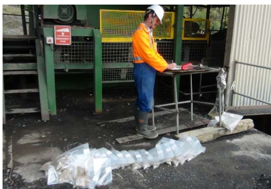
Ore being sampled as its being crushed
